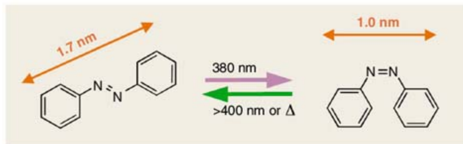
Fig. 2. Azobenzene photoisomerizes between an extended or trans configuration under visible light (left) and a bent or cis configuration under UV light (right), which is shorter by ~0.7 nm. \Delta indicates thermal energy.
